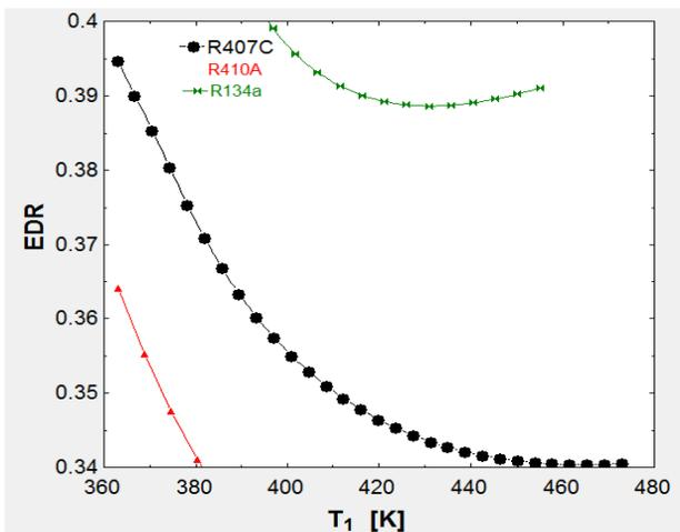
Figure 10: Variation of EDR with the inlet temperature of expander
