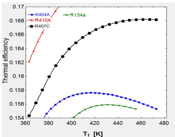
Figure 4: Variation of thermal efficiency of organic rankine cycle with expander inlet tempreature.
