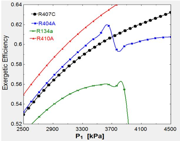
Figure 8: Variation of exergetic efficiency with the inlet pressure of expander
